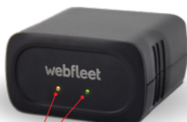
2 x LEDs for system and connection status
